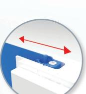
**SELF-ADJUSTING TRACKS** Fenetex tracks automatically apply proper tension to the screen. What looks like a one piece track is actually made of three aluminum extrusions. Two outer sections house a moveable inner section. The inner section moves with the screen while specifically designed springs maintain proper screen tension. The genius of the Fenetex system is that it eliminates any need for adjusting screws or magnets and is virtually maintenance-free.
